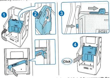
Lower the radio into the cradle and push down lightly to fully engage with the facility socket at the bottom of the cradle. The charging LED on the car kit will illuminate when the radio is correctly seated on the facility connector.
